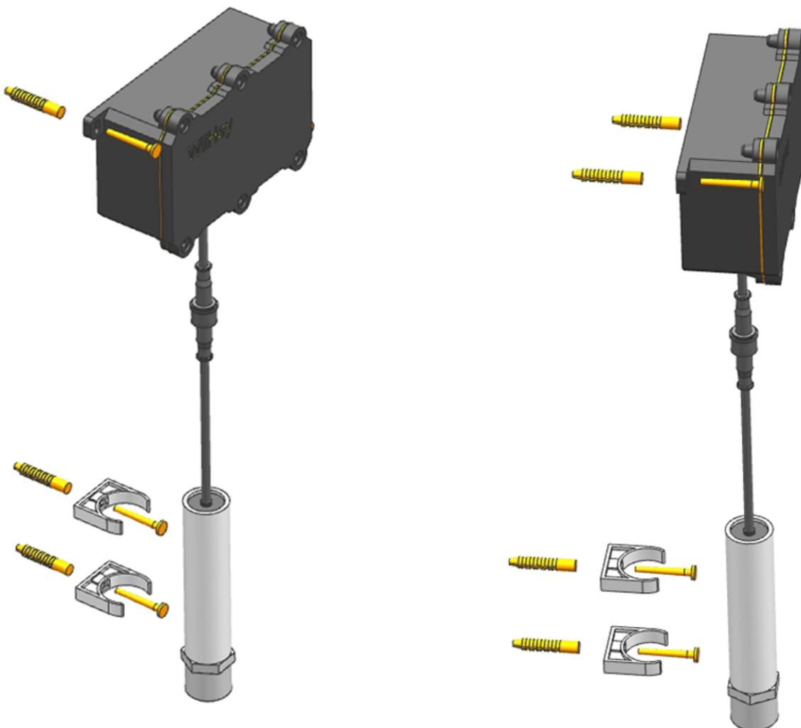
Use the wall pipe clamp directly on the wall as below
